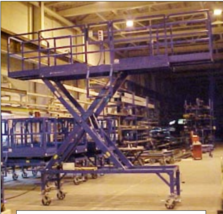
Above: Shown with Rollouts extended on each end, adding an additional 78" of platform length.
